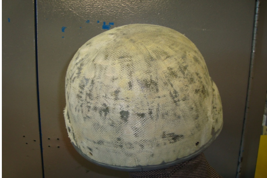
Figure 9: Damaged ACH after paint removal.
