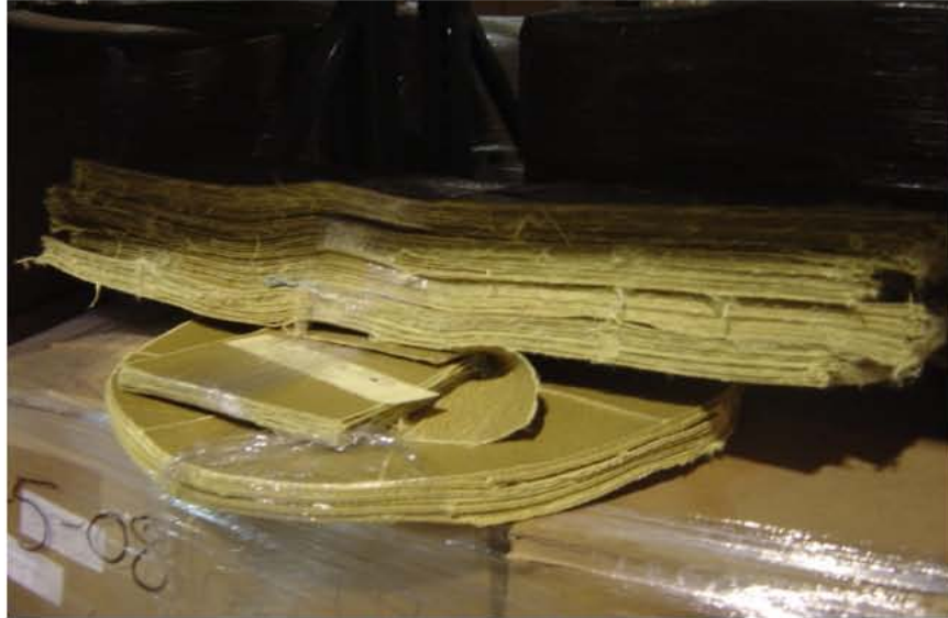
Figure 4: LMCH Kevlar bonded together.
