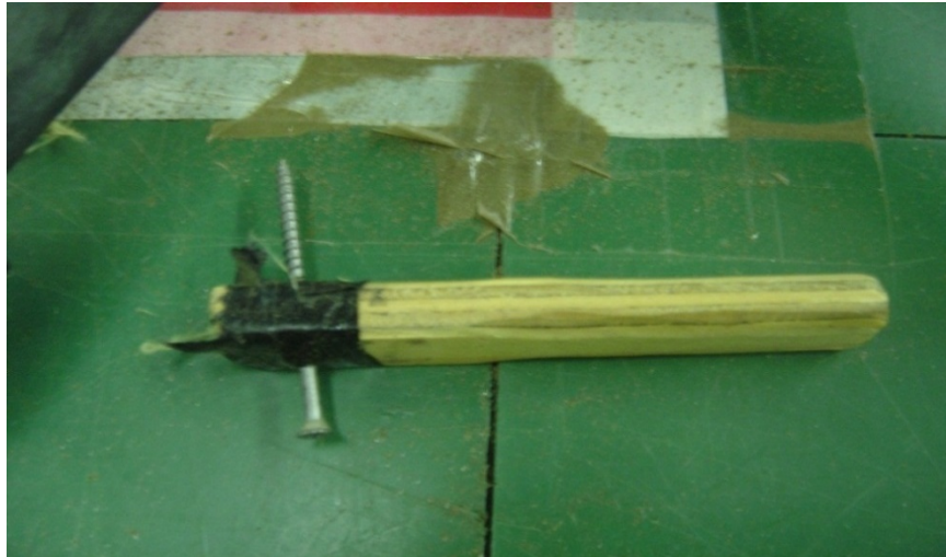
Figure 8: "Screw tool" used to strip Kevlar
