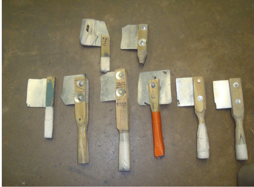
Figure 7: Hatchets used to remove paint.
