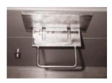
Insertion of used syringe in dispensing unit causes a new one to be released. Saxerriet Prison, Switzerland
