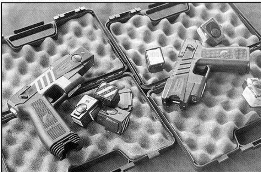
The 21-foot L.E. cartridges are quickly discerned from the 15-foot Civilian ones. L.E. is striped, civilian is solid yellow.
