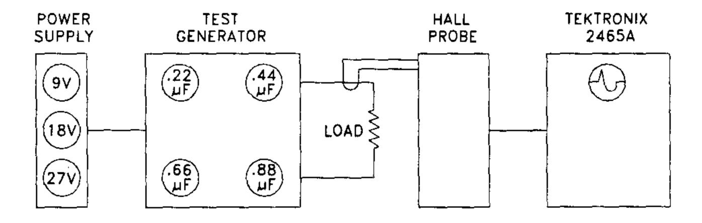
In addition to the familiar physical measurements of the pulse wave form using a 100 megahertz Tektronix 2465A Oscilloscope, a new high bandwidth Hall effect probe was used to accomplish indirect current measurements in the test circuits.
